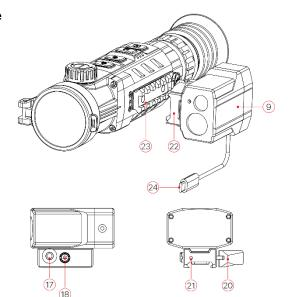
Connect the Type C plug (24) of the module to the Type C port (10) on the riflescope to finish the installation.
